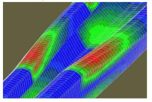
Compared with step 1 (stress of band edge) the profile stress analysis has the advantage that the longitudinal stress is calculated not only at the band edge but in the whole profile cross section. This is very important if maximum stress is not at the band edge, e.g. if folded edges are bent up.
